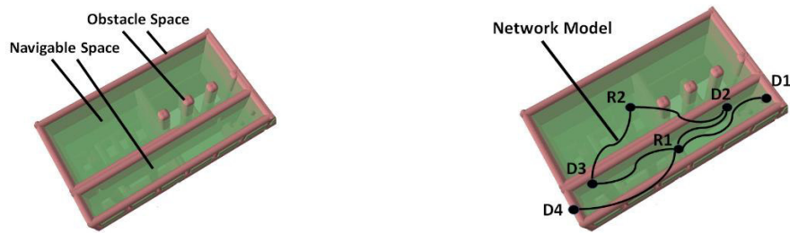
Fig.15. (A). Actual Navigable spaces after deducting obstacle spaces according to the wheelchair shown in green color (left). (B). Network model of the corresponding navigable space (right).
