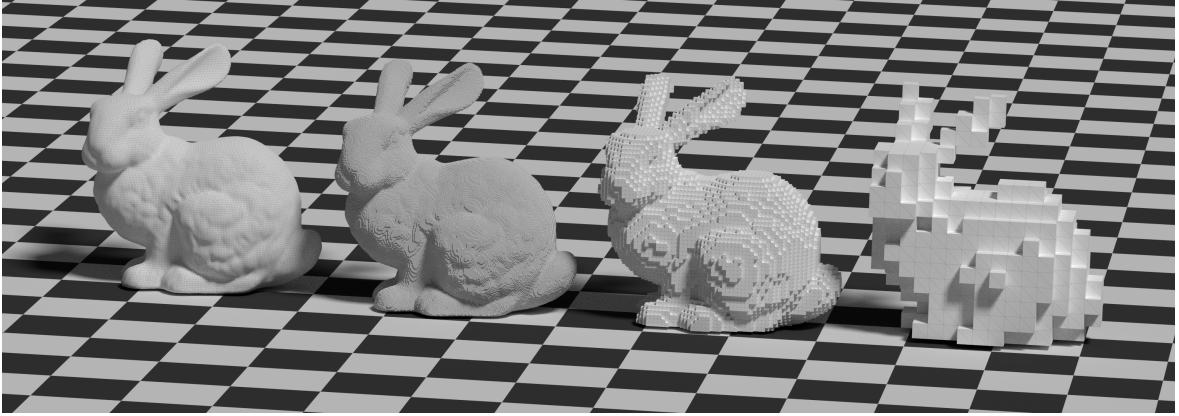
Figure 1: A voxelization of the Stanford Bunny dataset. On the left, the original input mesh, on the right, three voxelizations at different resolutions ( 256^3 , 64^3 and 16^3 ).
