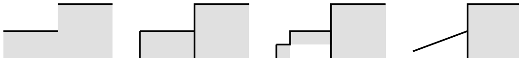
Figure 30: Transition between two blocks at different level-of-detail. On the left, the active faces are marked in black. Without any fixes, a gap may appear between the high- and low-resolution block. In the following two cases, the faces at the boundary have been closed using skirts, resolving the problem, even if the level-of-detail difference is higher than one. In the rightmost image, the left block has been refined to the source geometry, and the skirt ensures consistent rendering in this case as well.
