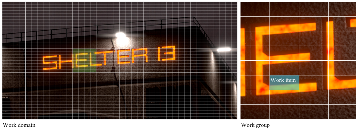
Figure 16: Work definition in OpenCL. On the left, the complete work domain (NDRange) is visible. It consists of multiple, independent work groups, as seen on the right. Each work group is comprised of multiple work items.
