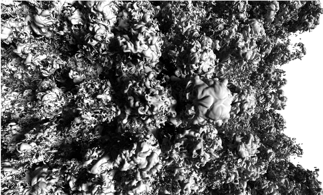
Figure 19: A voxel iso-surface extracted from the Richtmeyr-Meshkov instability at a resolution of 2048 \times 2048 \times 1920 voxels. The extracted surface consists of 128880391 voxels.
