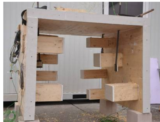
Figure 2: assembled specimen with measurement equipment before placed into the furnace
