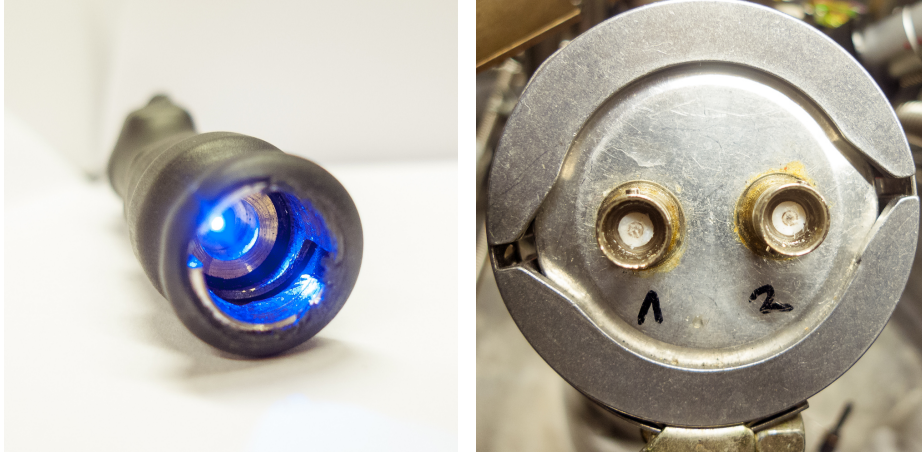
Figure 4.11: Image of the custom-made LED housing (left) and vacuum feed-through for the optical fibers (right). Then the feed-trough is sealed using Stycast 1266 epoxy resin.
