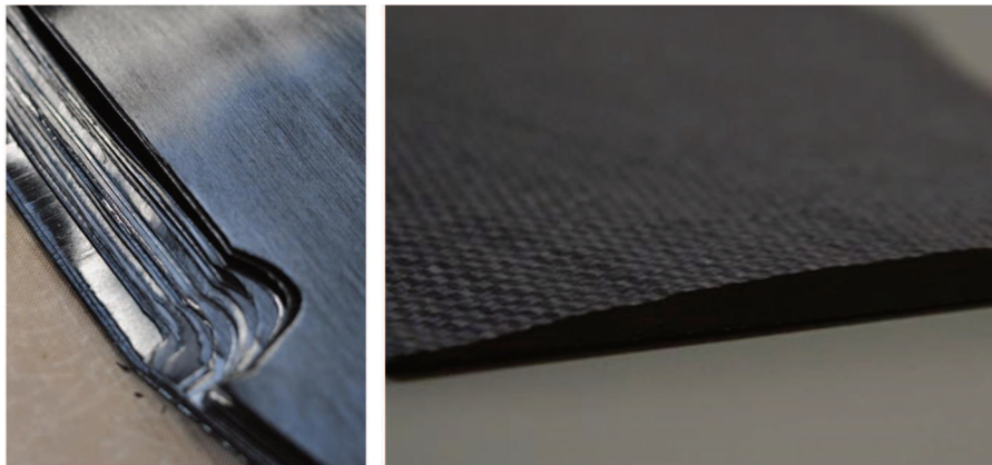
Figure 4.1 Preform stack before (left) and after (right) consolidation
