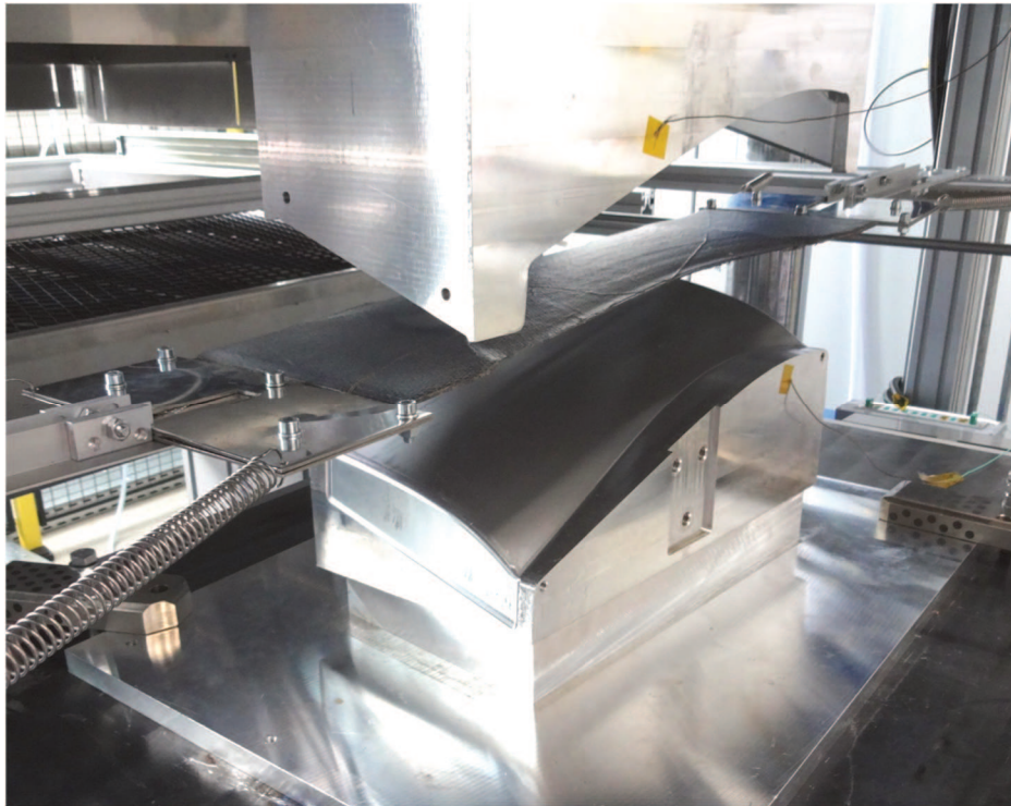
Figure 3.10 Organo sheet in press before thermoforming
