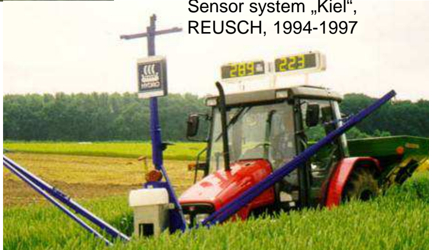
Mapping approach EM38 collecting soil data on-the-go
