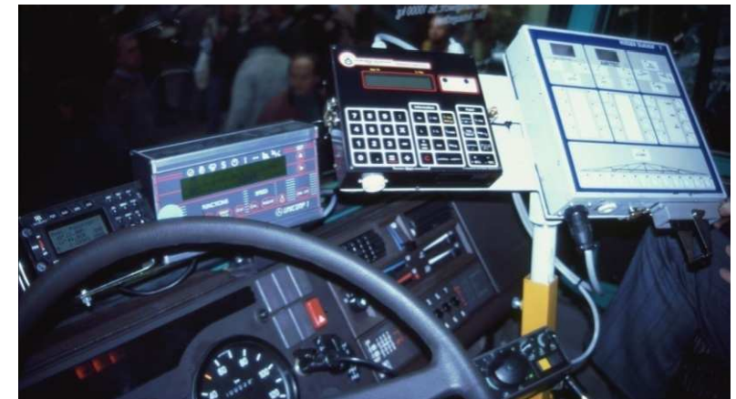
Non-standardized control of fertilizer spreaders by multi-purpose controllers
