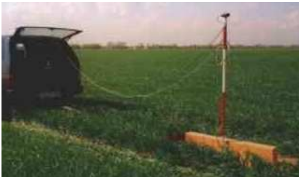
Mapping approach EM38 collecting soil data on-the-go
