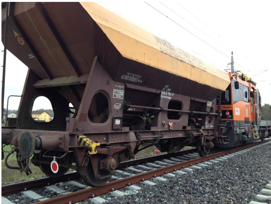
Pic 4: Ballast wagon for test of Benkelman beam and quasi-static test runs
