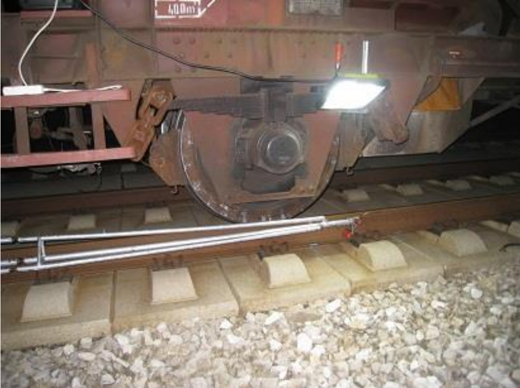
Pic 5: Benkelman beam test for elastic rail deflection (ballastless track)
