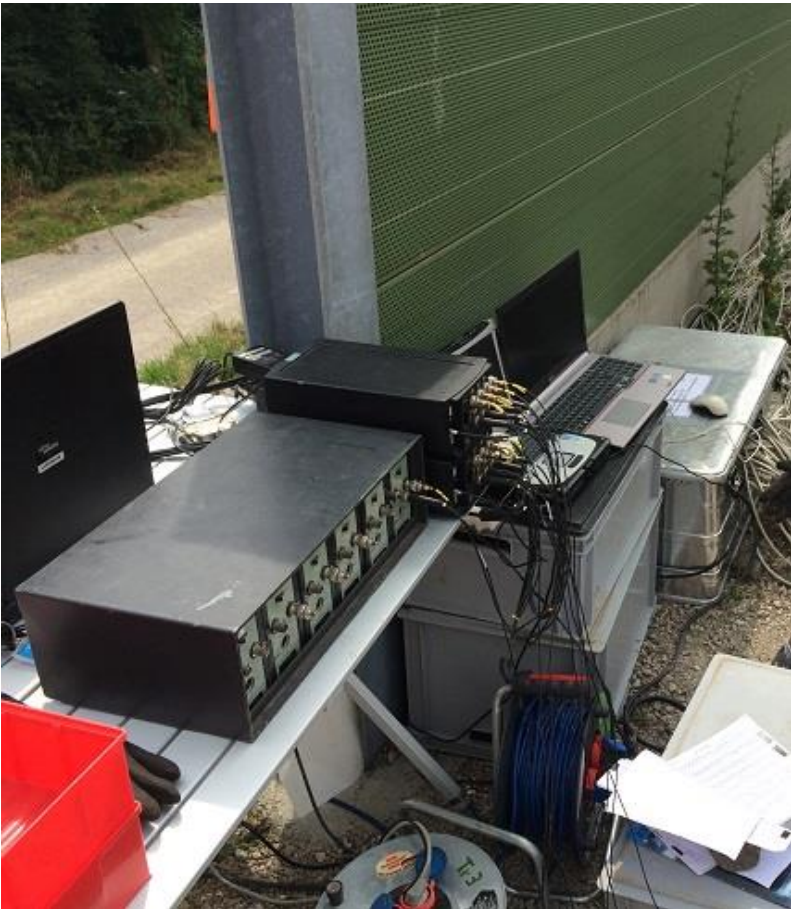
Pic 9: Built work station and data amplifiers for vibration measurement
