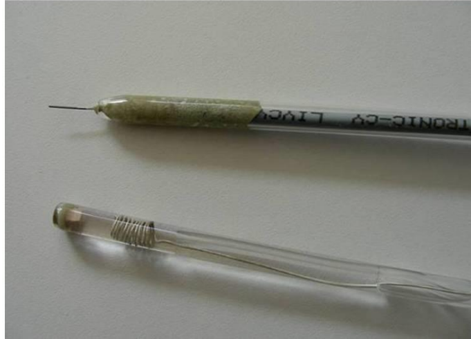
Figure A1: Eh sensor sensor pair for redox measurements. Schematic set-up (left) and picture (right) of the platinum electrode (top) and reference electrode (bottom)
