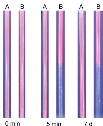
Fig. 7 Glass capillaries under 365 nm UV radiation, coated with A: SiNC-gPS (12 h polymerization time) and B: SiNCs hydrosilylated with 1-dodecene. The capillaries were half-immersed into 5 M aqueous KOH. 1-Dodecene functionalized SiNCs are dissolved by KOH, apparent by the disappearance of the photoluminescence, whereas SiNC-gPS are stable for more than a week under the given conditions.
