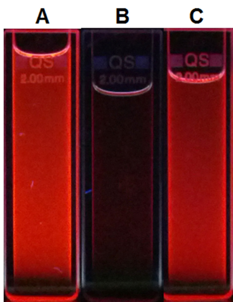
Figure S 4: Solutions of SiNC-SiCl functionalized with phenyllithium (A), lithium phenylacetylide (B) and (5-hexyl-2-thienyl)lithium (C) under 365 nm UV radiation.
