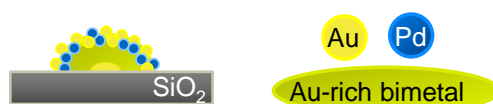
Figure 2.8. Schematic intersection of a PdAu particle on spent PdAu/SiO 2 with an Au enriched surface and a Pd enriched subsurface layer.
