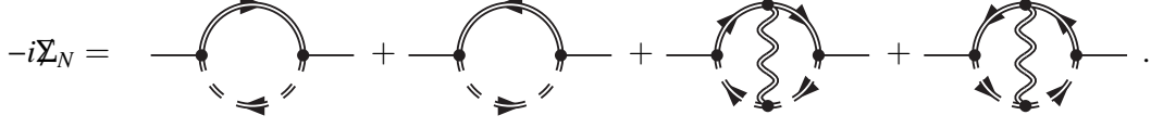
Figure 3.1: 2PI contributions to the neutrino production rate. Particles in the loops are left-handed leptons and Higgs, and the wavy line indicates U(1) and SU(2) gauge bosons. The double lines represent full propagators, and the external legs are understood to be amputated.
