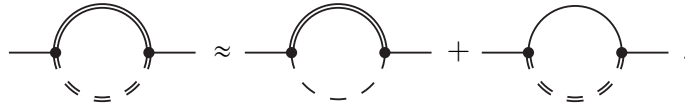
Figure 3.5: Expansion of the wv diagram according to Equation (3.31). Double and single lines indicate full and tree-level propagators, respectively. The charge-flow arrows are suppressed, but the sum of both cases is intended.
