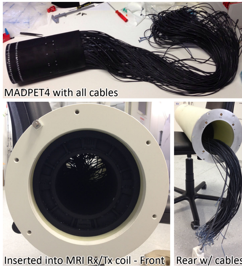
Figure 6.8.: Top: Final assembly of MADPET4 with all cables as tested inside the MRI. Left: MADPET4 inside the MRI Rx/Tx coil with the PET FOV matched to the coil's RF center. Right: Rear view of the Rx/Tx coil.
