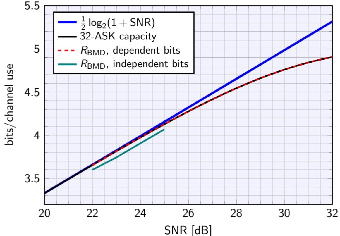
Probabilistic Amplitude Shaping with DVB-S2 Codes FER  $\leq 10^{-3}$
