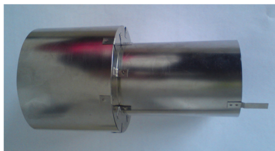
(b) Mumetal shielding with a thickness of 0.25 mm.
