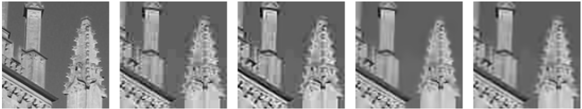
Figure 4.2: From left to right: Original image, JPEG-encoded image with quality value 12 (PSNR = 28.4 dB), DIP-deblocked image (PSNR = 27.8 dB), SA-DCT-deblocked image (PSNR = 29.2 dB), and REAPP-deblocked image (PSNR = 28.9 dB).
