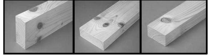
Figure 5. Presence of defects (knots) in a timber element
