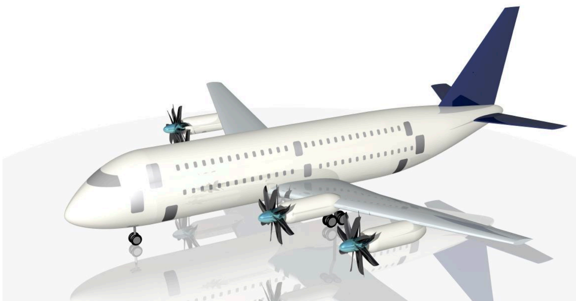
Figure 1.2: Computer aided design visualization of the developed high-capacity aircraft concept for short- to medium-range operations (Iwanizki 2013)
