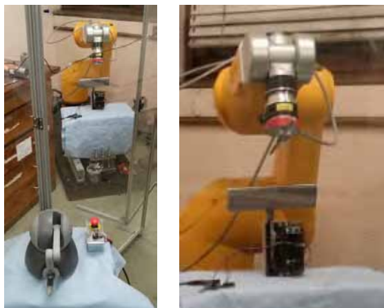
Fig. 3 Picture of the hardware setup on the left, with the Phantom Omni master in the foreground and the Stäubli TX90 slave in the background. The picture on the right shows the setup of the oscillating surface, seen as a grey foam block on the bench under the Stäubli TX90 tool.
