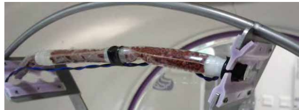
Fig. 5 The Core-Snake inside a Labcaire Autoscope ISIS Automated Endoscope Reprocessor.
