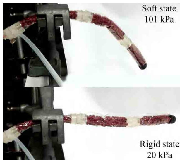
Fig. 3 The snake bending due to weight when soft (top) vs the snake holding a horizontal position when rigid (bottom).
