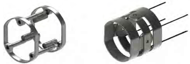
Fig. 2 CAD models of kinematic module: parallel (l.) and serial (without prismatic joint) (r.) configuration
