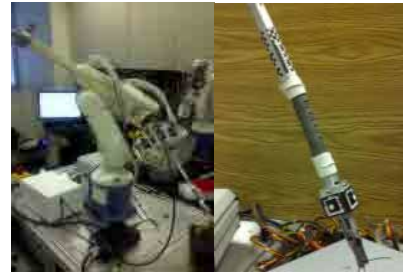
Fig. 2 Left: Robotic arm, Right: Anastomosis tool
