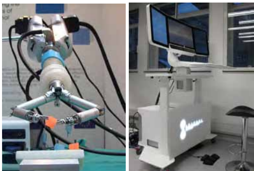
Fig. 1 The upgraded version of the SPRINT system: (Left) robotic platform and (Right) the console (developed at the Hamlyn Centre for Robotic Surgery by Prof. Guang-Zhong Yang).
