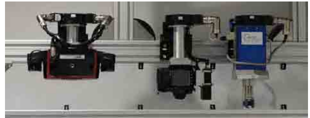
Fig. 1 Virtobot tool magazine. From left to right: 3D surface scanner, digital SLR camera, biopsy tool.
