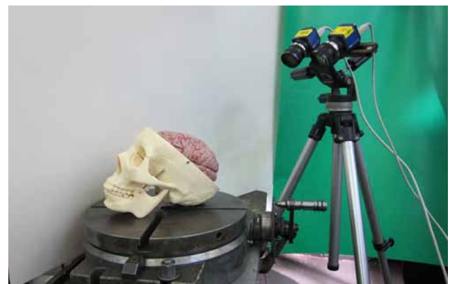
Fig. 2 Photograph of the experimental setup. The stereo cameras are mounted on a tripod (left) and point to the plastic brain model, mounted on a Cartesian displacement table.
