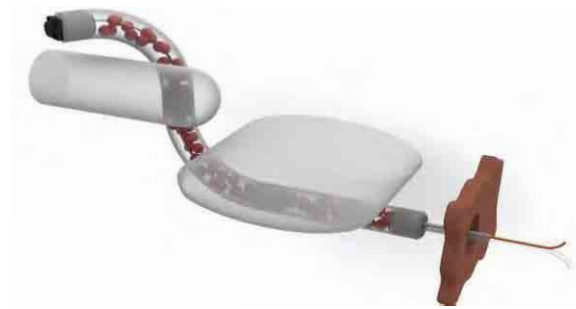
Fig. 1 The Core-Snake, a low cost, granular jamming-based flexible laparoscopic camera. Shown here its ability to access difficult areas, while occupying 4 mm of trocar port space.
