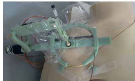
Fig. 3 First prototype of the robot with ABS material mounted on a body phantom. A protective cover is used to separate disposable part from the rest of the robot.
