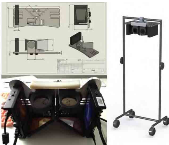
Fig. 1 CAD design, stereoscopic viewer unmounted and suspended from stand.
