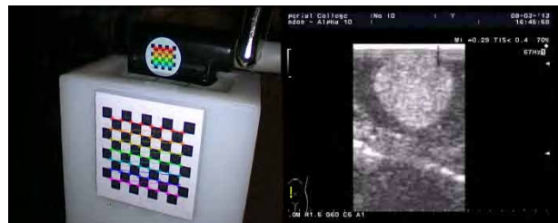
Fig. 2 Ultrasound image acquisition (left-to-right): probe calibration using water-filled Z-phantom and dual pattern technique; and typical ultrasound slice showing subsurface extent of phantom tumour.
