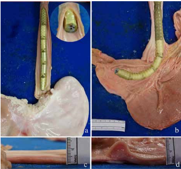
Fig. 1 Ex-vivo porcine upper gastro-intestinal specimens with a) oesophagus detubularised and b) stomach transected in mid-coronal plane, demonstrating procedural configurations of the i-Snake® for POEM and POEP respectively. Thickness of luminal muscle layers were 3mm, 4mm and 10mm for the c) oesophagus, d) stomach and pylorus respectively.
