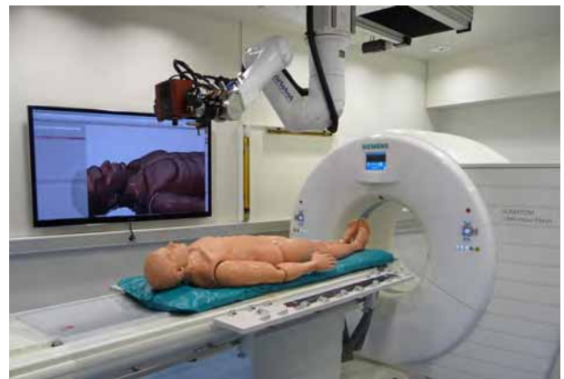
Fig. 2 Virtobot arm equipped with 3D surface scanner.
