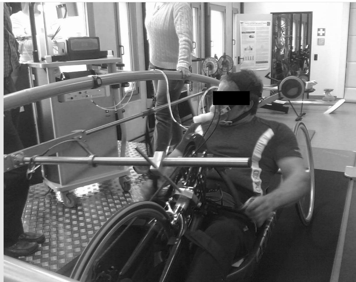
*Figure 1. Paraplegic athlete during incremental step test with Handbike mounted on treadmill.*
