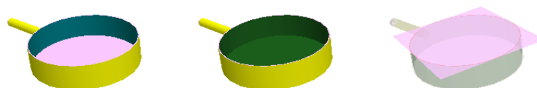
Figure 6.18: A cooking pot segmented into primitives. The second image shows the container marked as dark green. The last image shows the fit plane for upper edge.
