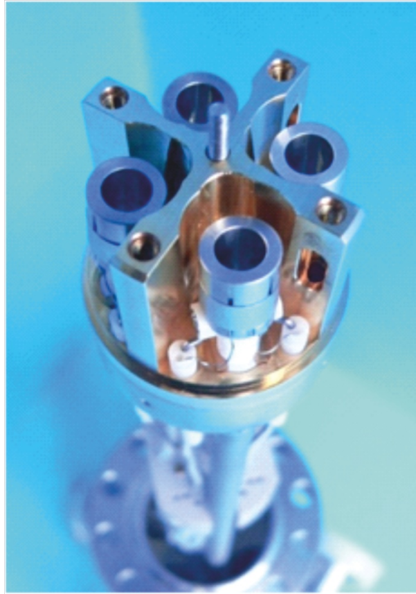
Figure 2 . 14 | OMBE showing the four crucibles containing molecules
