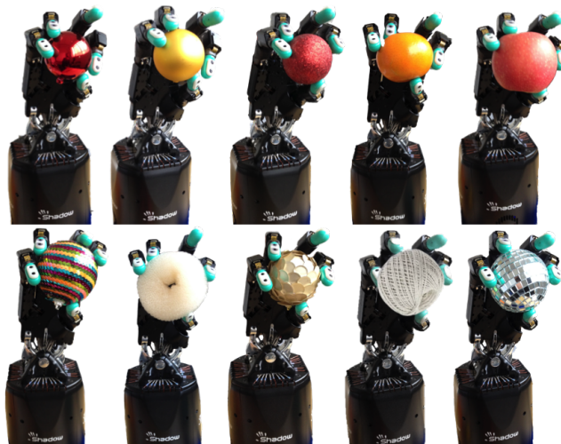
Fig. 1. The Shadow Hand is exploring the texture properties of the in-hand objects with an identical shape. It moves any of the fingertips to slide over the objects surface.
