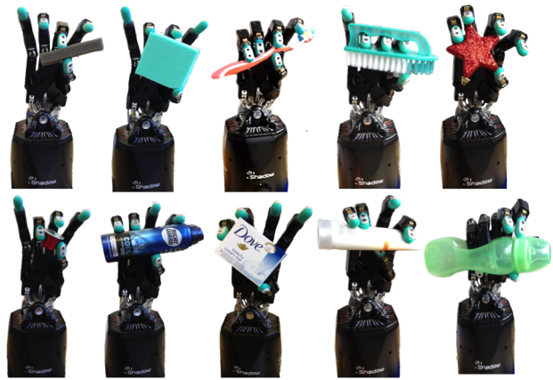
Fig. 3. The Shadow Hand is exploring the texture properties of the in-hand objects with complex shapes. It moves any of the fingertips to slide over the objects surface.
