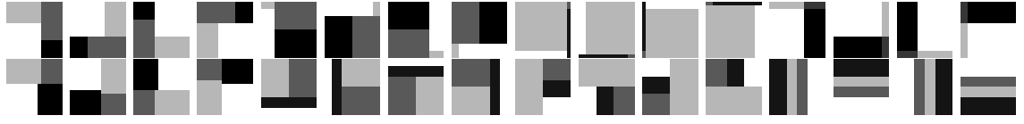
Figure 7.6.: Construction of the group pattern. Each image visualizes one basic group configuration for a 8 \times 8 signal. Larger group patterns are generated by combining the depicted group blocks and randomly assigning the different groups.
