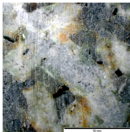
Fig. 63: Flossenbürg: granite under reflected-light microscope.
