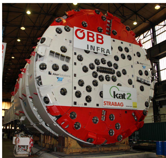
Fig. 39: Cutterhead design of Aker Wirth doubleshield TBMs used at KAT2 (www-03; mod. from ÖBB-INFRA 2009a).
