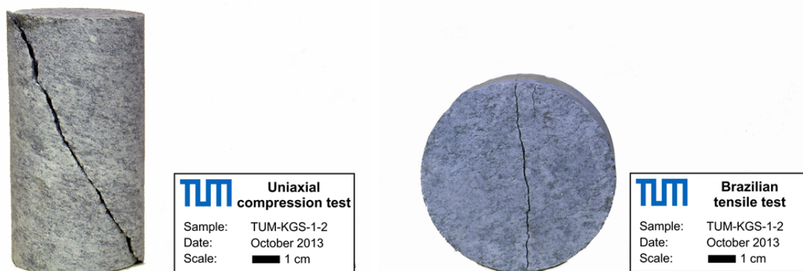
Fig. 22: Rock specimens of calcareous mica schist as representative of a tough rock type after uniaxial compression testing and Brazilian tensile testing. The ratio of UCS and BTS can be used to classify rock toughness.
