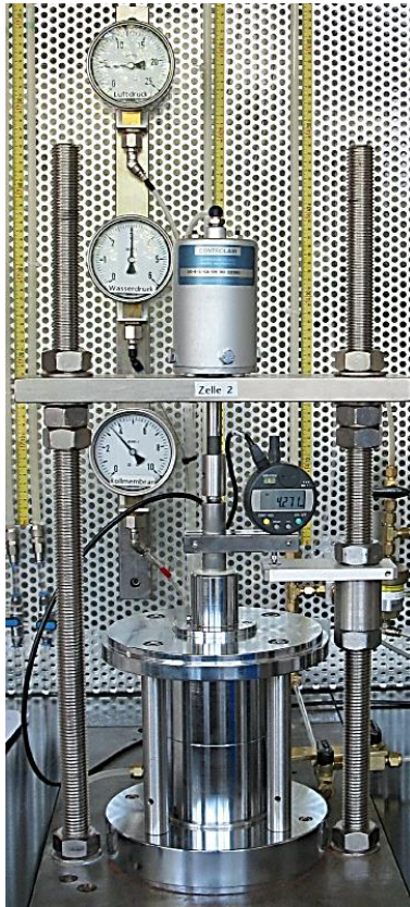
Figure 3.18. TUM-cell (Cell 2) which was built by the Zentrum Geotechnik, Technische Universität München.
