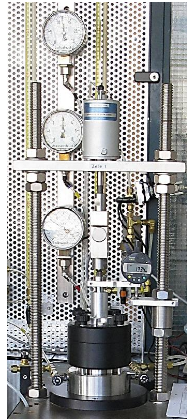
Figure 3.19. Wille-cell (Cell 1) built by Wille Geotechnik in collaboration with Prof. Schanz (as cited in Birle, 2011).
