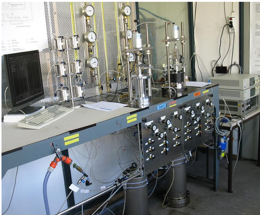
Figure 3.17. The suction-controlled oedometers that were used in this study (Zentrum Geotechnik, Technische Universität München).
