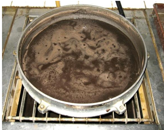
Figure A.1. Appearance of a light brown foam during the wet sieving (Zentrum Geotechnik, Technische Universität München).
