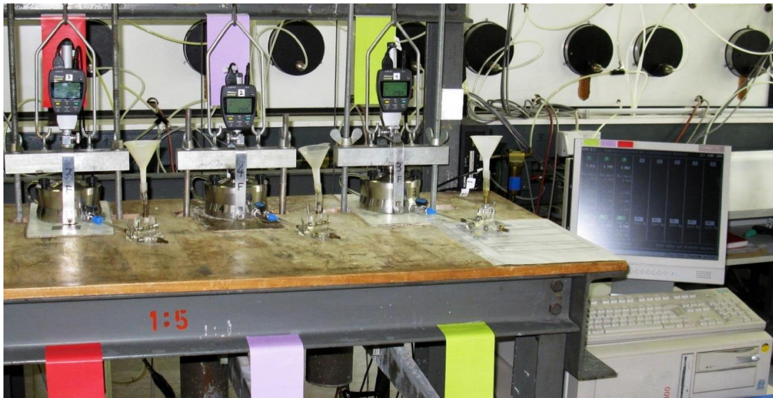
Figure A.7. Conventional oedometer apparatus used in this study for Tests S1, S2 and S3 on saturated soil samples (Zentrum Geotechnik, Technische Universität München).
