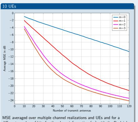
different number of bits for the phase information (m) with the Rayleigh channel model
