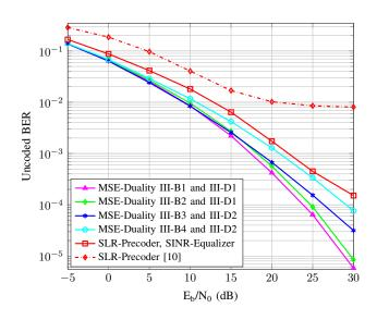
Figure 1. BER of the two iterative designs for  $N_t = 4$ ,  $N_r = 2$  and U = 2.
