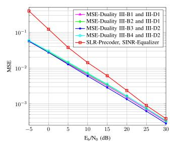
Figure 2. MSE of the two iterative designs for  $N_t = 4$ ,  $N_r = 2$  and U = 2.
