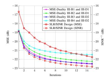
Figure 3. Algorithm convergence at  $E_b/N_0 = 5dB$  of the iterative designs for  $N_t = 4$ ,  $N_r = 2$  and U = 2.
