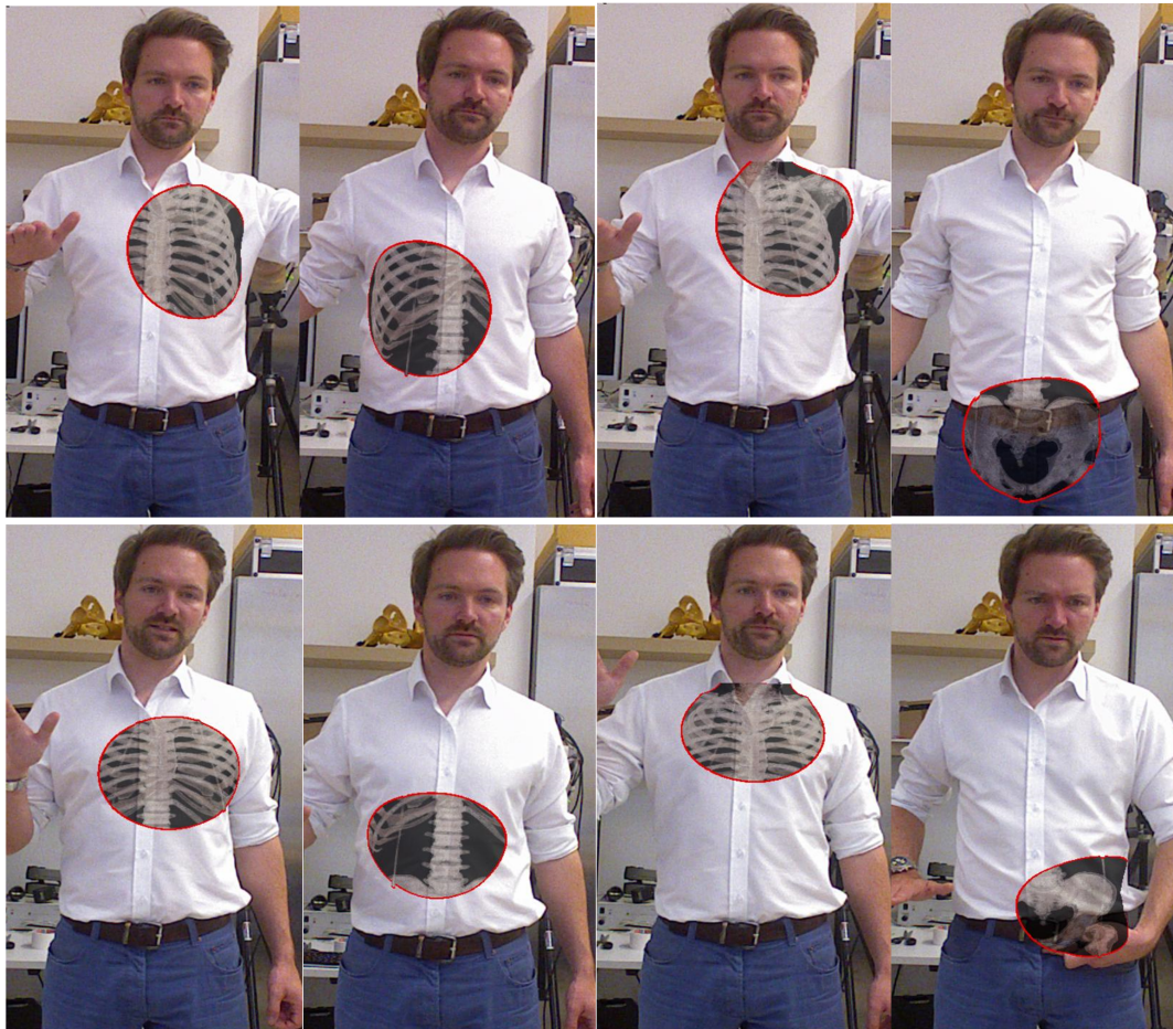
Figure 3.13 The Magic Mirror before (top) and after (bottom) the Kinect skeleton adjustment. Column 2 depicts the bottom of the rib cage being positioned correctly after skeleton correction.
