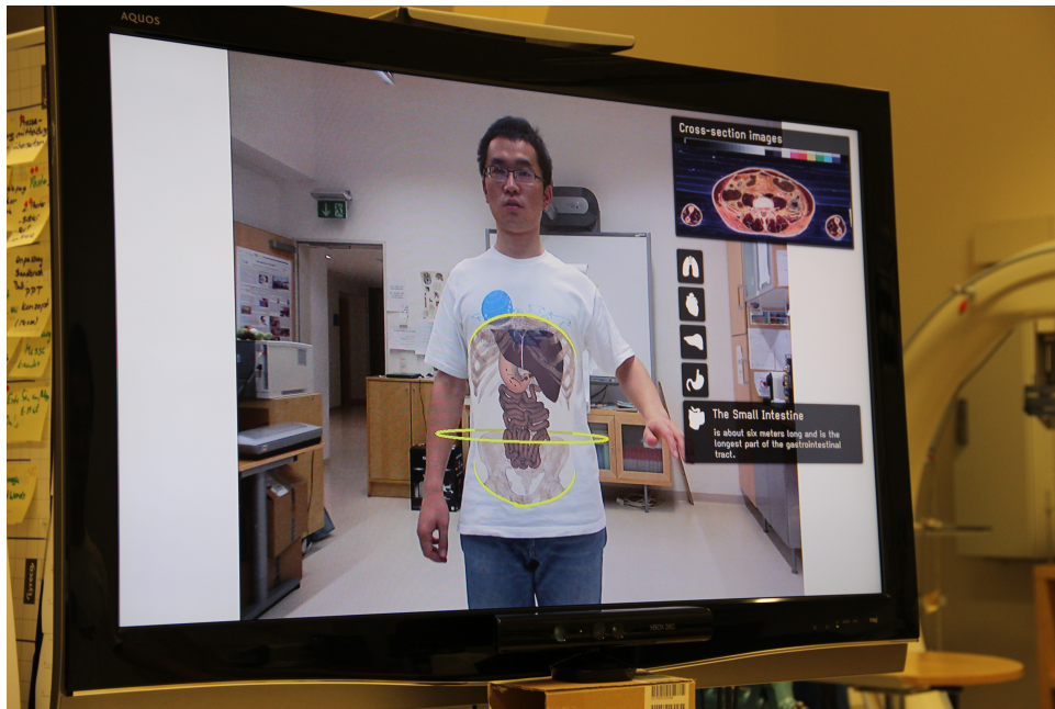
Figure 3.1 The system prototype has a mirror-like effect to the user by projecting a “looking glass” on the body. By using the Magic Mirror metaphor, the user is led to believe that he or she is able to look inside their own body.
