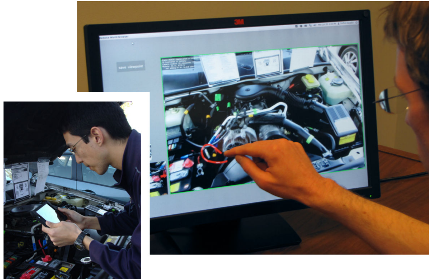
Figure 2.14 In touch with the remote world. A remote user points out an element in the environment (here: a car's engine bay) by drawing an outline around it. The annotation is world-stabilized and displayed in augmented reality to the local user (bottom left), who is holding a tablet.
