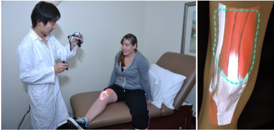
Figure 2.6 AnatOnMe in use in a simulated physical therapy consultation. The physical therapist explains a knee injury to his patient using on-body projection of medical imagery.
