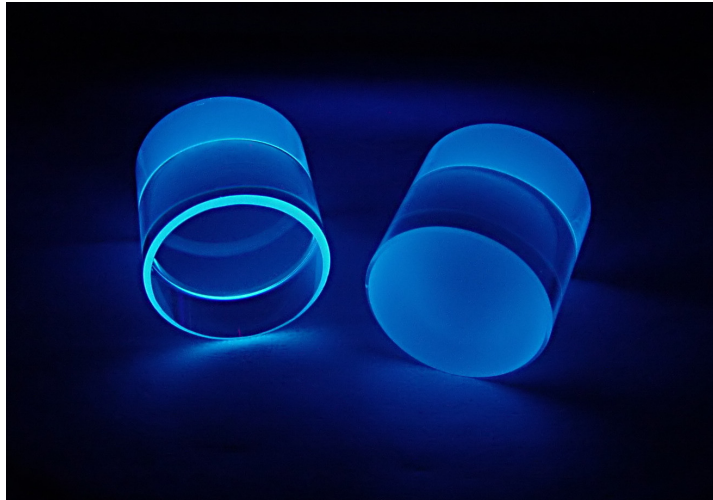
Figure 3.2: Two cylindrically shaped \text{CaWO}_4 crystals ( \varnothing = h = 40 mm, m = 300 g) are irradiated with UV light. The plane surface of the right crystal facing the observer is roughened to increase the probability for scintillation light escaping the crystal. Furthermore, the light output is more homogeneous than for the crystal with the polished surface (left), where it is concentrated at the baffled edges.
