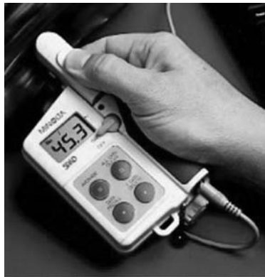
Figure 4 SPAD-Meter (by courtesy of YARA GmbH & Co. KG, Dülmen, Germany). (For colour information, please see the colour plate section.)
