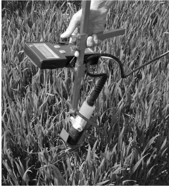
Figure 9 Hand-held fluorescence sensor (by courtesy of Fritzmeier Umwelttechnik GmbH & Co., Germany).
