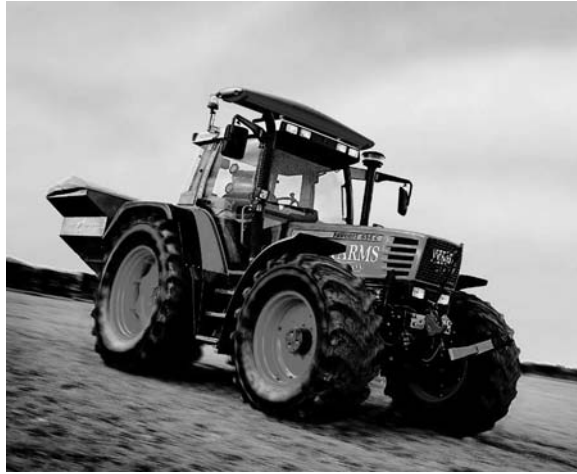
Figure 8 N-Sensor on tractor roof (by courtesy of YARA GmbH & Co. KG, Dülmen, Germany). (For colour information, please see the colour plate section.)
