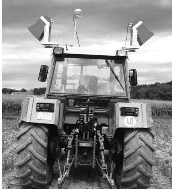
Figure 11 Laser-induced chlorophyll fluorescence sensor Planto N-Sensor (Planto GmbH, Leipzig, Germany, by courtesy of Technical University of Munich). (For colour information, please see the colour plate section.)
