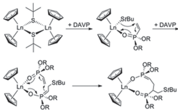
Figure 8. Initiation and propagation of DAVP polymerization via thiolato initiators.
