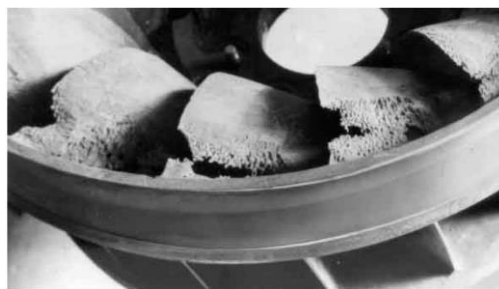
FIG. 2.8 Damage on the blades at the discharge from a Francis turbine. Reprint with permission from Ref. 4. Copyright 1994 by C. E. Brennen.
