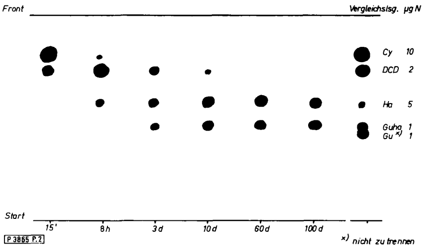
Abbildung 2: Cyanamid-Abbau in Gegenwart von amorphem Fe(III)-hydroxid Cyanamide breakdown in the presence of amorphous iron(III)-hydroxide
