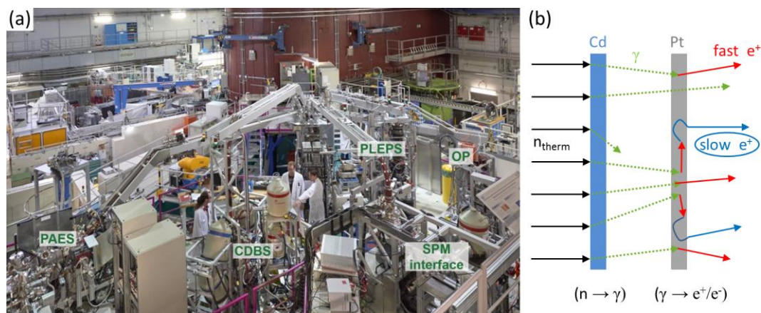
Figure 3.18: (a) Photo of the positron beam facility and instrumentation at NEPOMUC (FRM II): PAES (positron-induced Auger-electron spectrometer), CDBS (coincident Doppler broadening spectrometer), PLEPS (pulsed low-energy positron system), SPM interface (scanning positron microscope), and OP (multi-purpose open beam port). 107 (b) Principle of neutron-induced positron formation at NEPOMUC. 108
