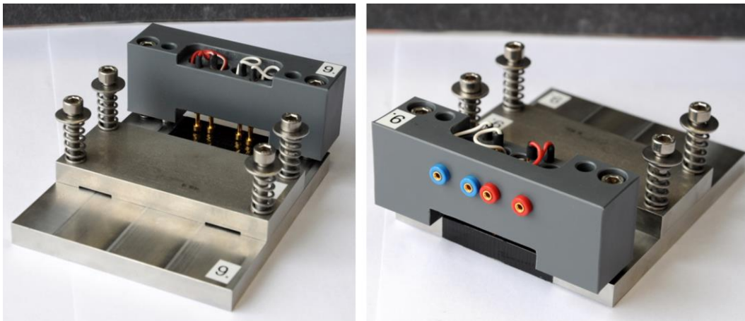
Figure 4.50: Photos of the special-designed pouch-cell compression tool with adjustable spring pressure. The loading can be adjusted between 0.15 and 0.2 MPa.
