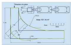
The curve intersection line was used as comparative measurement of the tractrices, being based on the length of the bisectors from the point of intersection of both outer edges of the road through to the inner tractrix line. These curve intersections measured 2.67 m for the tractor with plough, 7.72 m for tractor with tandem trailer, 8.41 m for the agricultural trailer combination, 6.69 m for the beet harvester and 7.40 m for the combine harvester.
