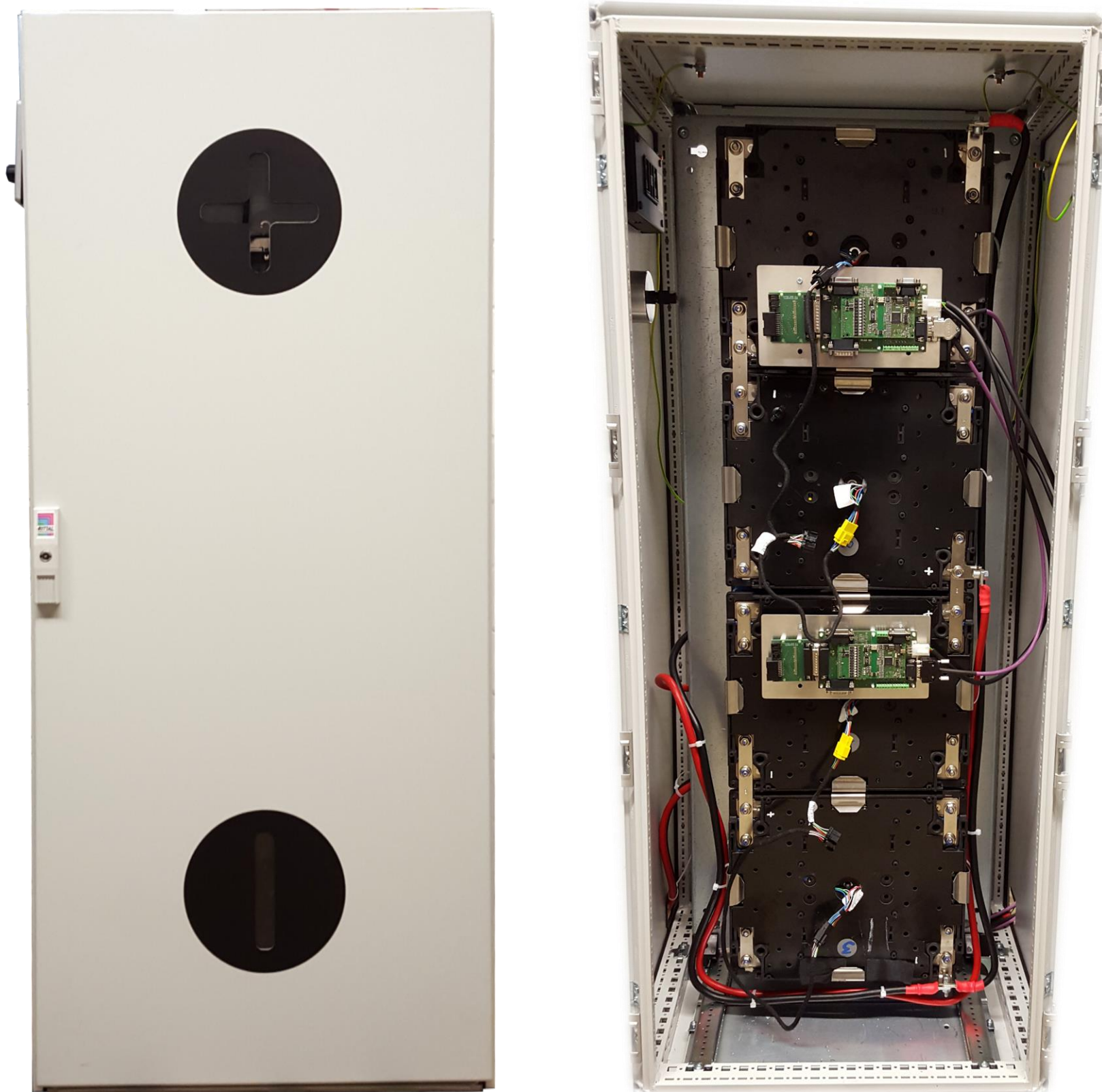
Fig. 1: The developed second life stationary storage system (left) and its internals (right)
