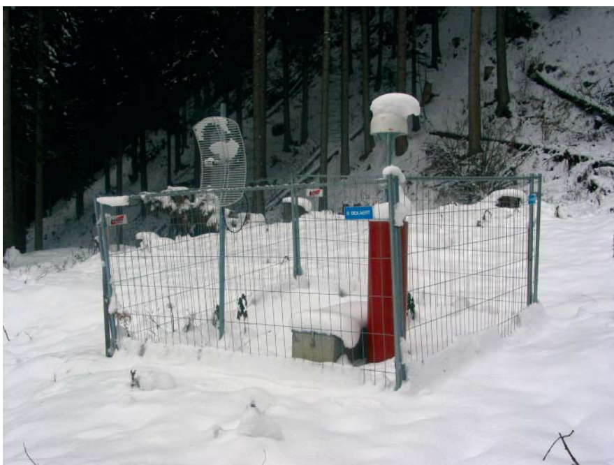
Figure 4: GPS point 'Plateau' with tiltmeter and WLAN antenna.
