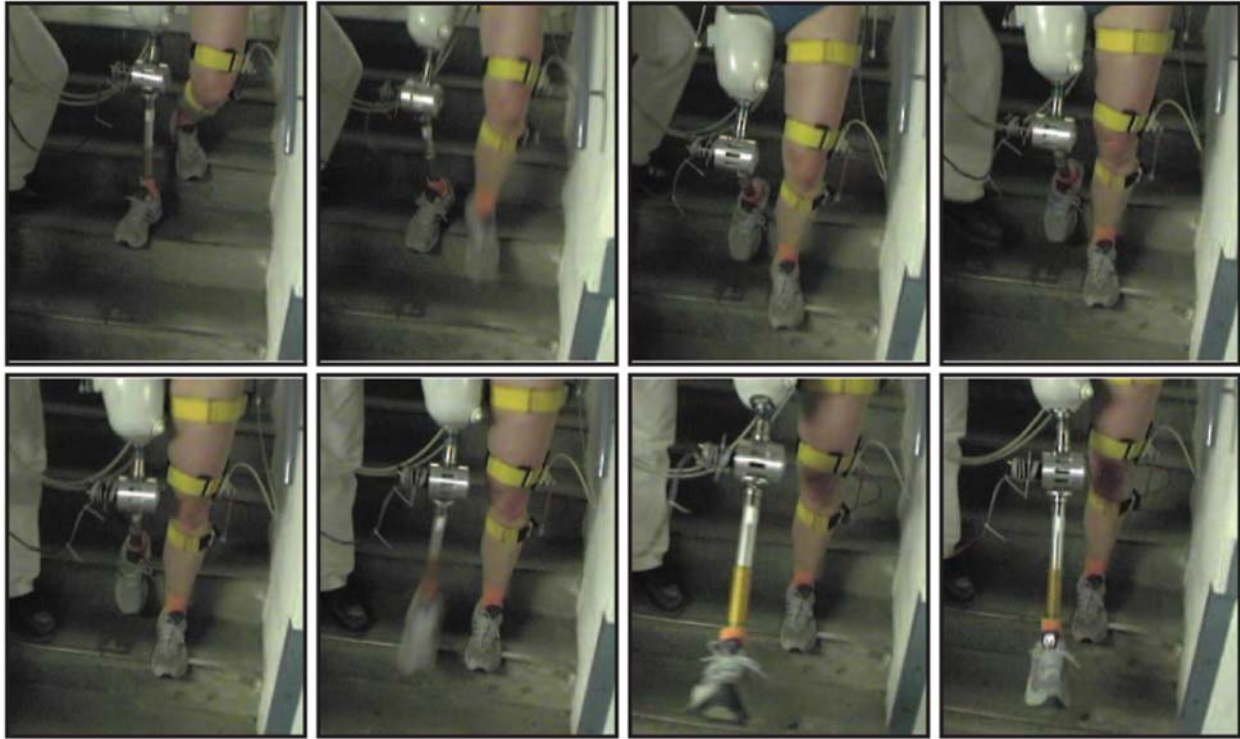
Figure 6 Stair descent with a CLME-controlled prosthetic knee joint. An assisting person (left) helps with balance. Time between adjacent frames: 40 ms.
