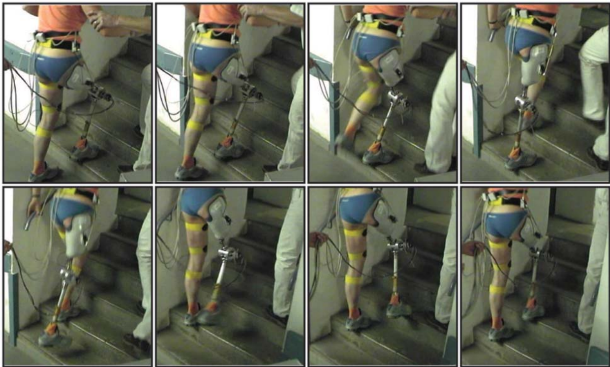
Figure 5 Stair ascent with a CLME-controlled prosthetic knee joint. An assisting person (right) helps with balance. Time between adjacent frames: 40 ms.
