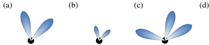
Figure 5.8: Lobular glyphs of a (a) bimodal and (c) trimodal PDF, with lobe lengths given by weights after normalization by the maximum weight. (b),(d) Lobular glyphs without weight normalization are considerably more difficult to distinguish.
