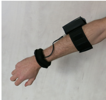
Figure C.5: The vibrotactile wristband consisting of a band of stretchy fabric in order to ensure user comfort.
