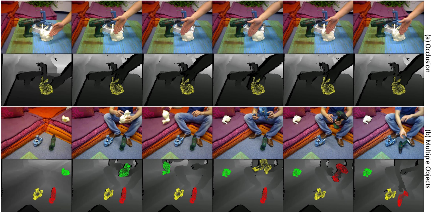
Figure 5.9: Qualitative results of the (a) robustness to occlusion and (b) scalability to track multiple objects.
