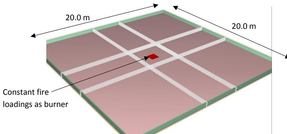
*Image 2* Geometry of 2<sup>nd</sup> model in planned real-scale simulation (\*the top slab of 8 cm concrete slabs with/without ventilation openings are hidden for illustration purposes)
