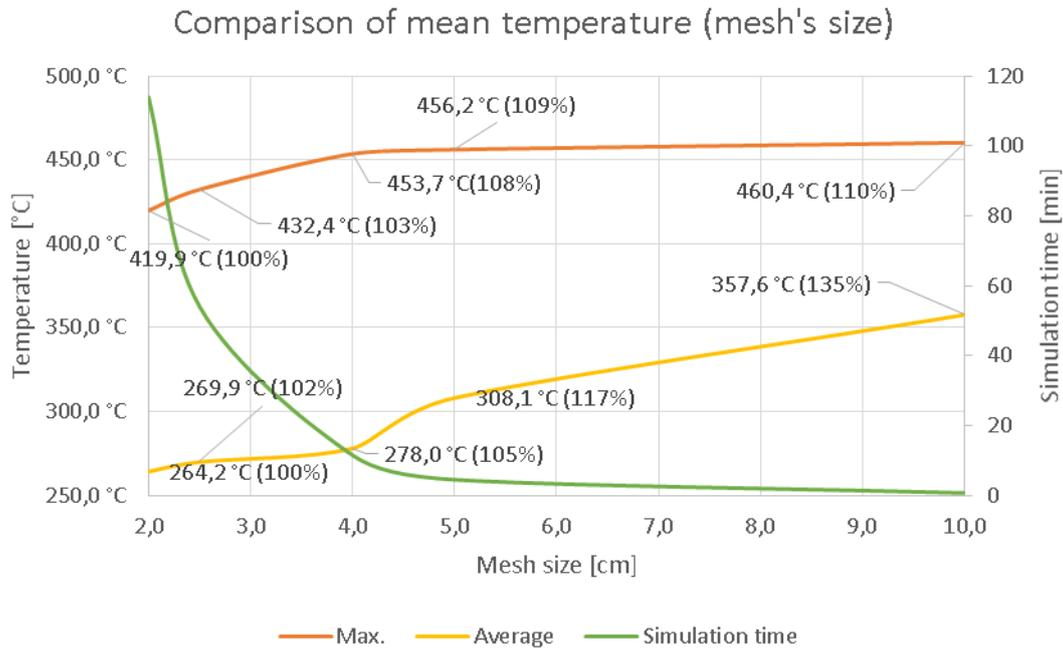
*Image 6 Comparison of max and average mean temperature as well as simulation time, depending on the mesh size*
