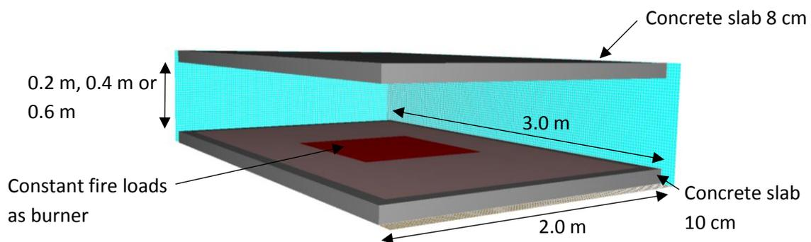
*Image 1* Geometry of 1<sup>st</sup> model in bench-scale simulation (\*the outer walls of 8 cm calcium silicate panels with ventilation openings are hidden for illustration purposes)
