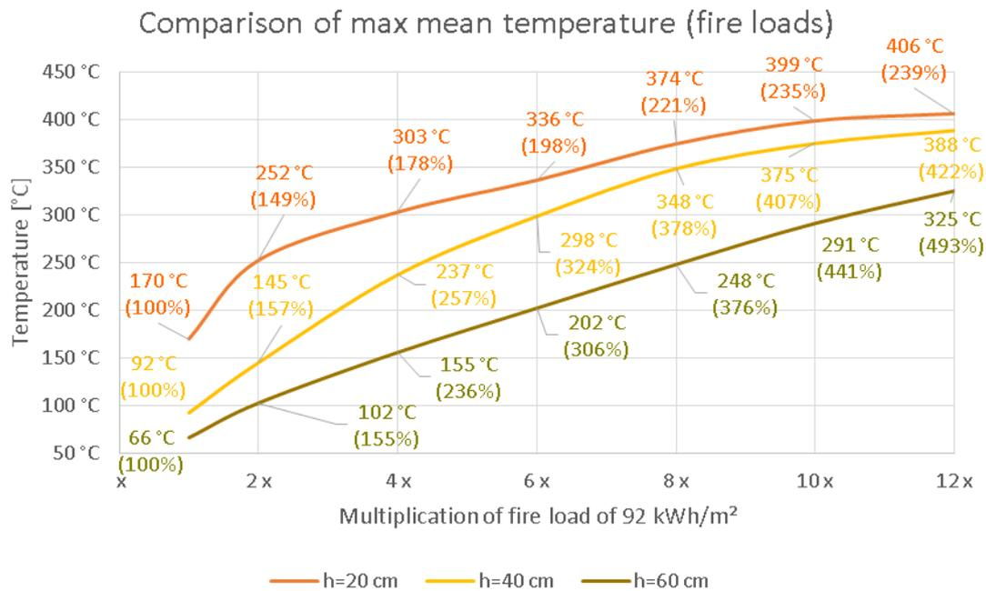
Image 4 Comparison of max mean temperature, depending on the fire loads for hollow spaces with a clear height of 20 cm, 40 cm and 60 cm.
