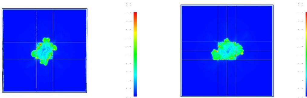
Image 9 Temperature distribution for 9 and 13 mesh divisions for 2<sup>nd</sup> model with a base area of 20 m x 20 m. [Left: 9 divisions and right: 13 divisions]
