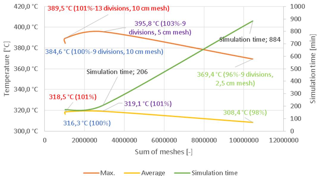
Image 8 Comparison of max and average mean temperature as well as simulation time, depending on number of cores and outer mesh size. The fire mesh size remains at all time at 2.5 cm.
