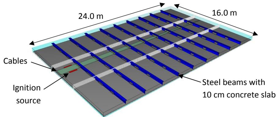
*Image 3 Initial geometry of 3<sup>rd</sup> model with clear height of 39.5 cm in future simulation (\*the top slabs and side walls are hidden for illustration purposes) (Simulation is modelled after [2])*
