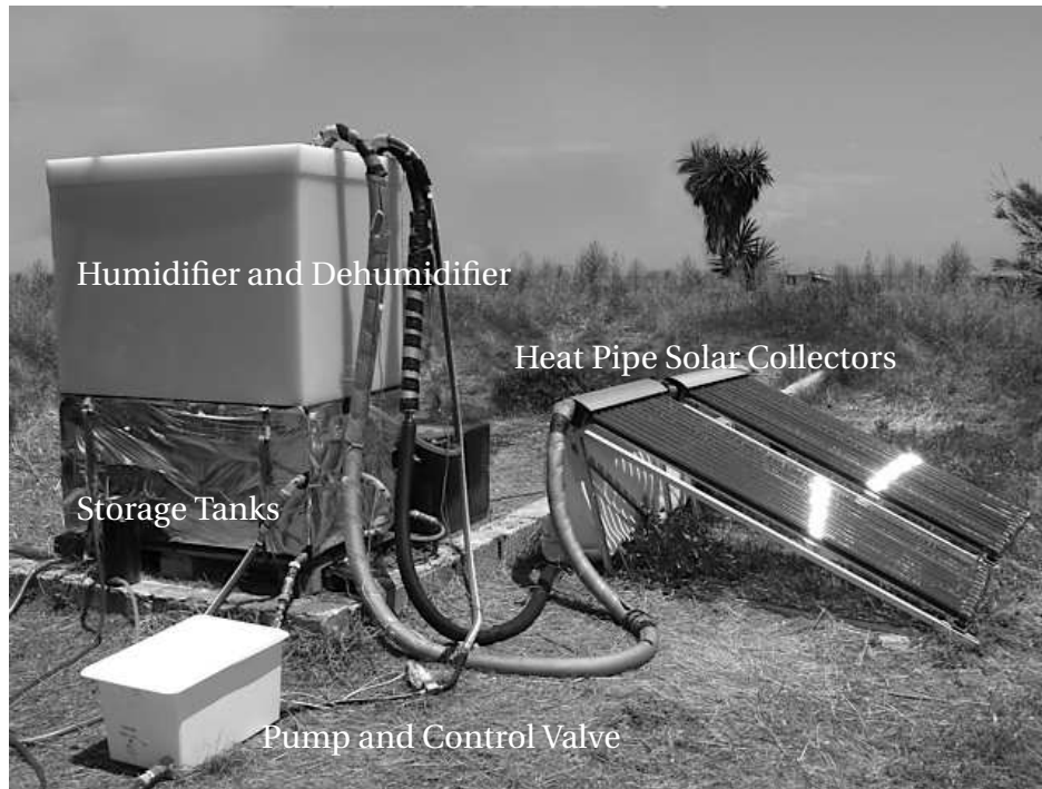
Figure 5.3: Field Test of Solar Powered Single-Stage HD System in Corfu, Greece
