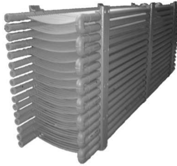
Figure 5.6: Dehumidifier for Singe-Stage Experimental HD Setup; Total Surface Area: 5.8\text{ m}^2
