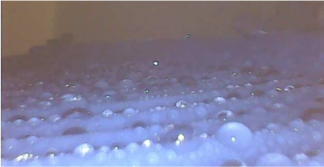
Figure 5.7: Dropwise Condensation on the Top Layer of the Tubular Polypropylene Heat Exchanger Surface of the HD Single-Stage Setup ( t_{A,deh,in} \approx 75\text{ °C} , t_{W,deh,out} = 68\text{ °C} , d_{tube} = 4.5\text{ mm} )
