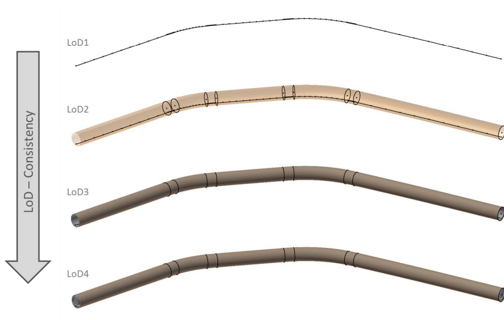
Figure 61: Multi-scale tunnel model represented up to the fourth LoD. Due to the top-down design approach and the loose dependency system established among geometric objects, multi-scale product models become very sensitive to geometric inconsistencies between LoD.
