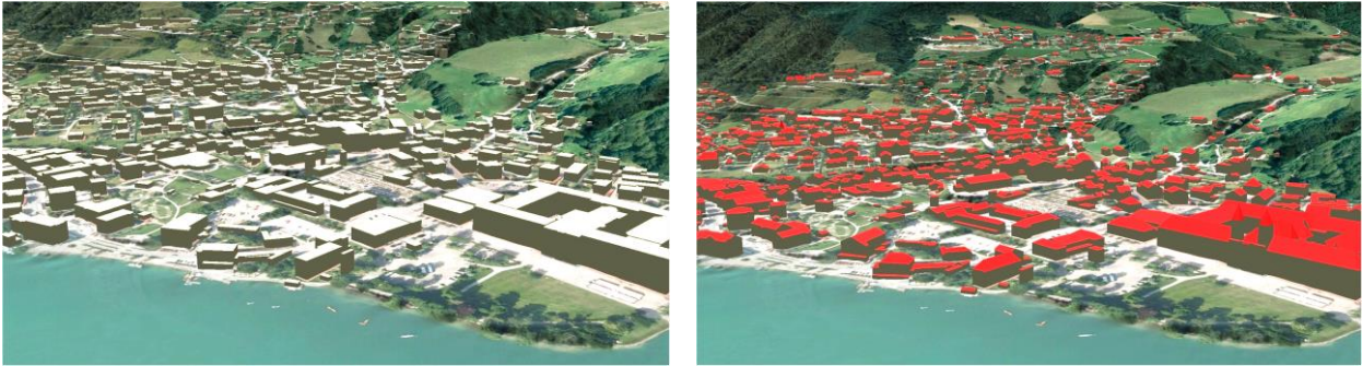
Figure 2-5: Buildings: left) LOD 1, right) LOD 2
