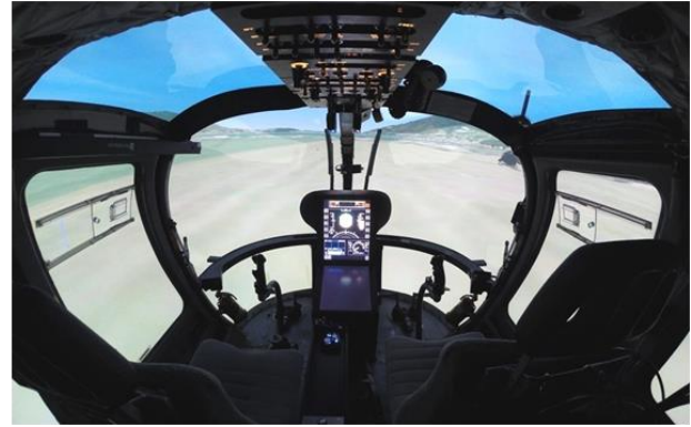
Figure 4-7: Cockpit: 2 display configuration
