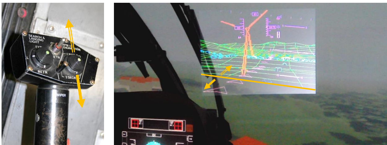
Figure 4-21: Near-field culling adjustment with a switch at the collective stick
