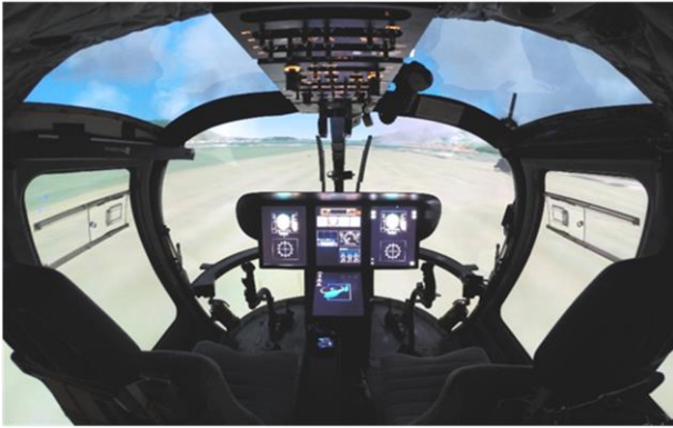
Figure 4-6: Cockpit: 4 display configuration
