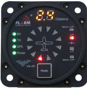
Figure 2-12: FLARM – collision avoidance system [8]
