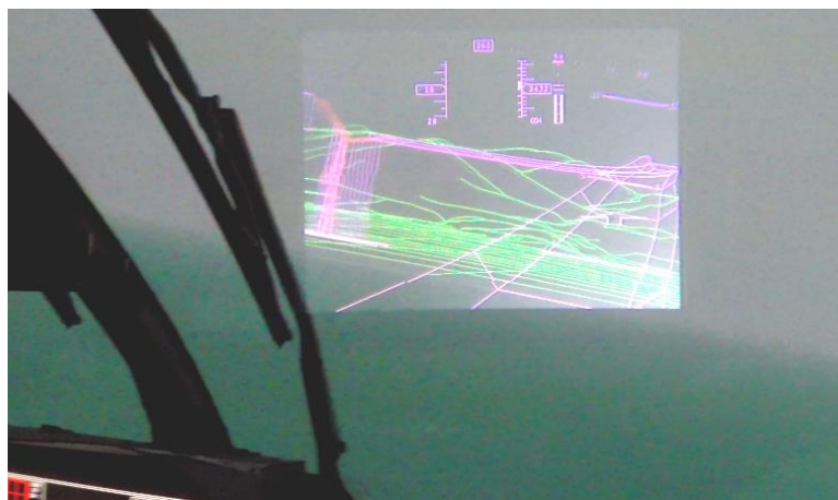
Figure 4-25: Highway-in-the-sky in bathtub style for wind turbine approach
