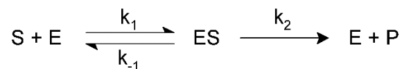
Figure 3.8 – Reaction scheme of an irreversible reaction with one substrate S and one product P. The substrate binds to the enzyme E forming the enzyme-substrate complex ES. The substrate may either dissociate from the enzyme in its unchanged state or be converted to the product before dissociation. The constants k denote the rate constants of each step.
