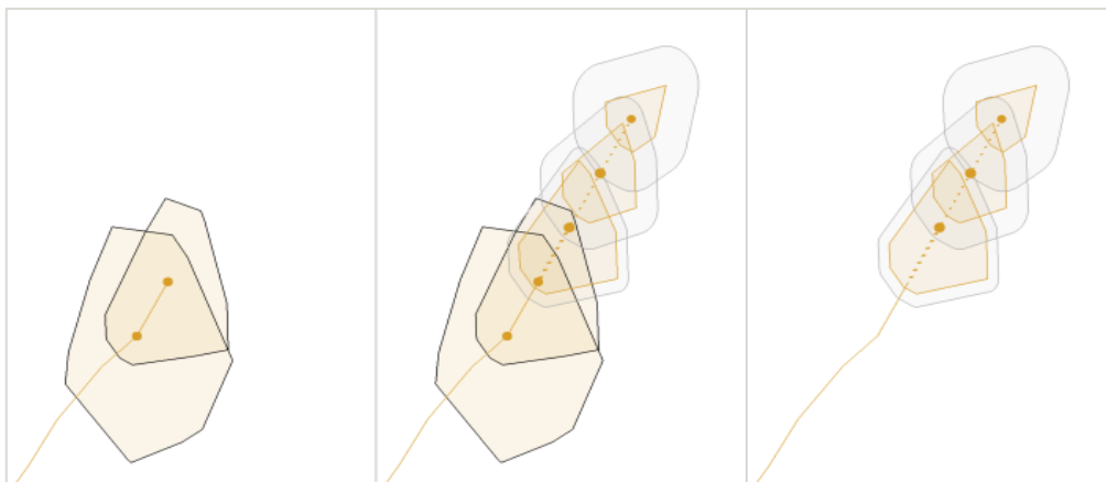
Figure 5. Buffered prediction uncertainty of nowcasting: last two lightning clusters (left), predicted clusters (right); past and predicted clusters (middle) (Peters, 2014)
