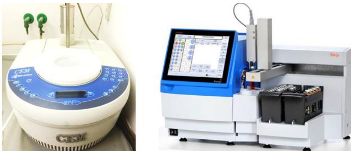
Figure 41. CEM Focused Microwave (left) and Biotage Initiator Robot (right) as applied in the thesis.
