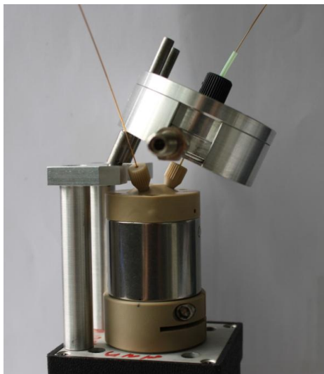
Figure 16: Valve, Equipped with Detection Cell, Cell Housing, and Cell Mount.
