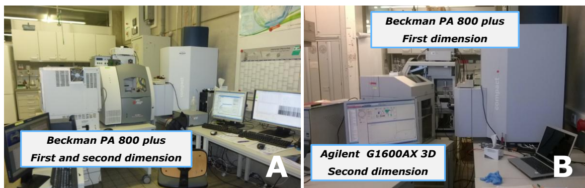
Figure 43 A-B: Comparison of the two 2D Setups using A: The Beckman PA 800 plus for Both Dimension in Combination with the HV Power Supply of the Beckman P/ACE MDQ Instrument, and B: using the Beckman PA 800 plus only for the First and the Agilent G1600AX 3D for the Second Dimension.
