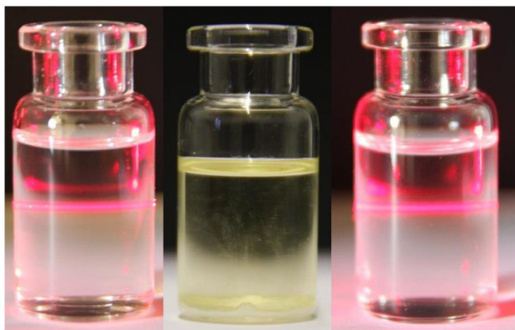
Figure 3—Tyndall effect of sodium zirconium lactate (left) and zirconium triethanolamine (right) complexes solved in DI water. Center: Precipitation of ZrO_2 from the solution of zirconium triethanolamine in alcohol.
